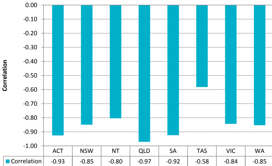
Figure 5-9 Correlation of net cost and installed capacity of PV excluding rushed buying periods
