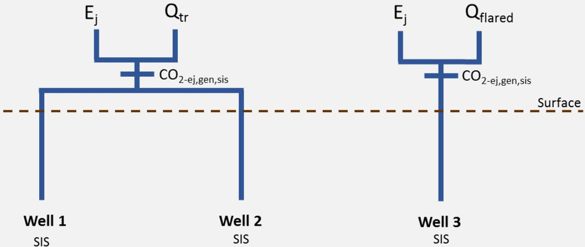
In this example, three 'Surface in seam' wells drain coal mine waste gas to the surface.
