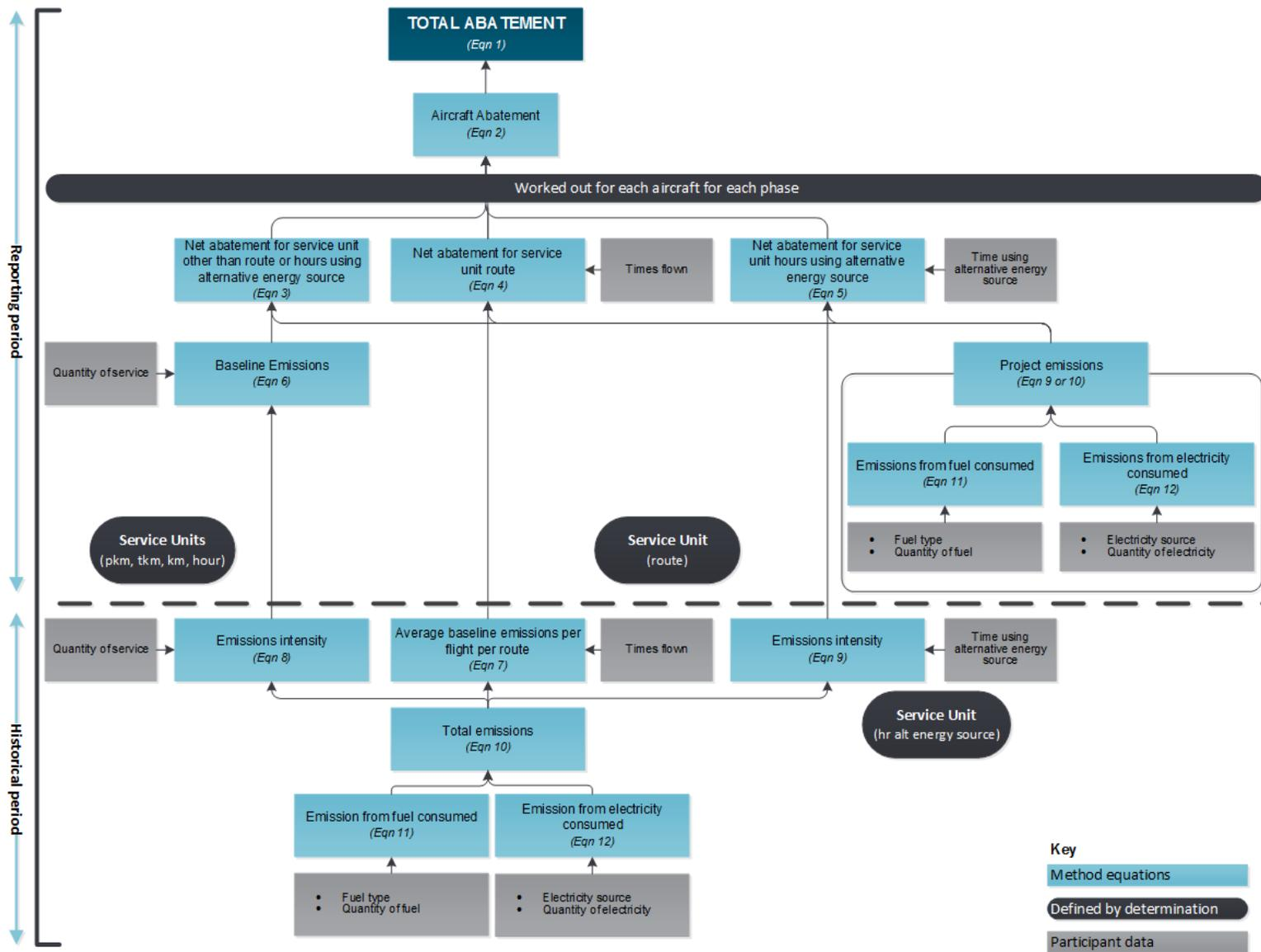
Figure 2 – Aviation method equation flow chart
