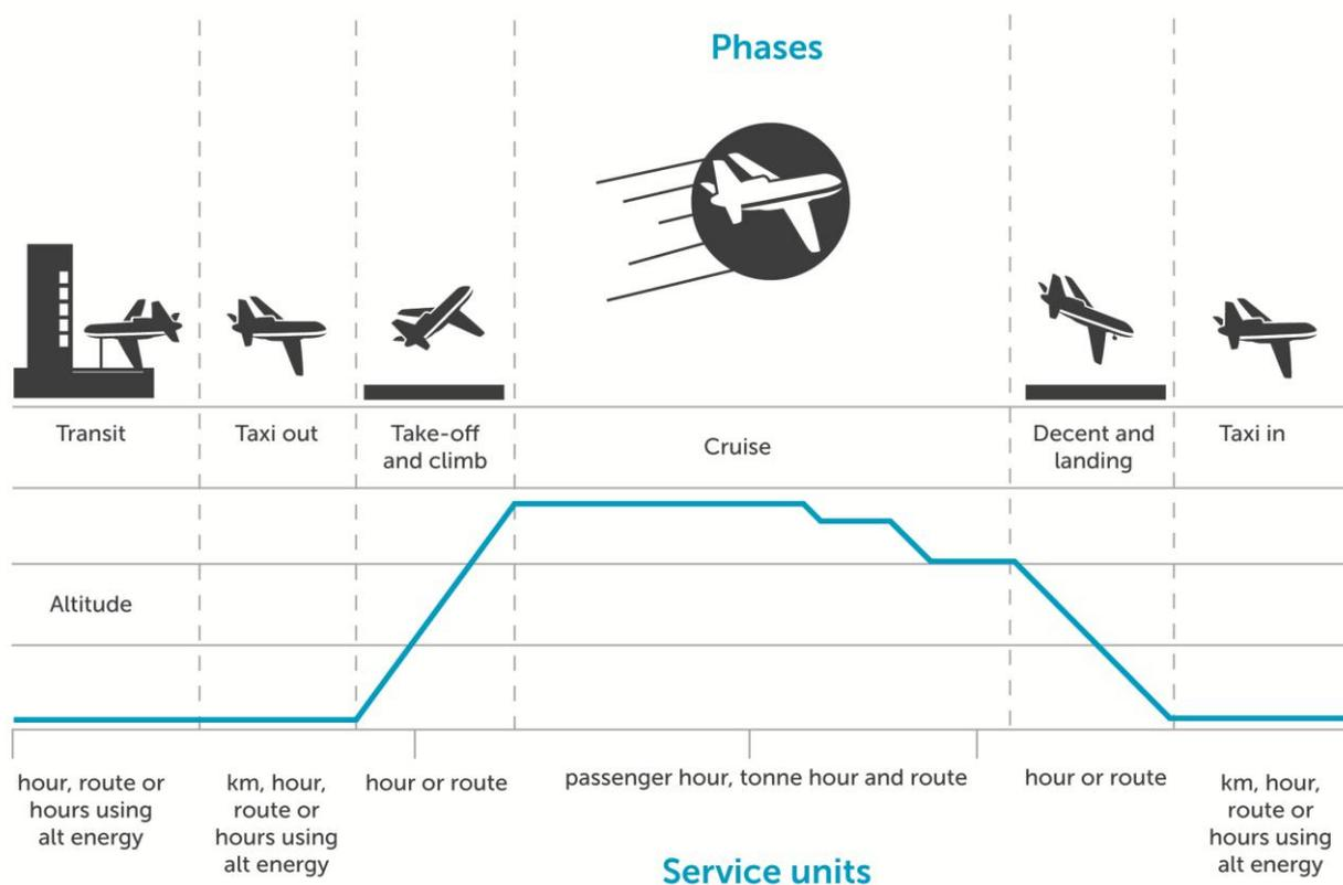
**Figure 1: Phases of aircraft operation and service units**
