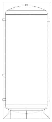
**Figure A1.** Large hot water tank resting on a ring that supports the tank on the ground. The inside of the supporting ring contains air, which substitutes for the insulation on the tank underside.
