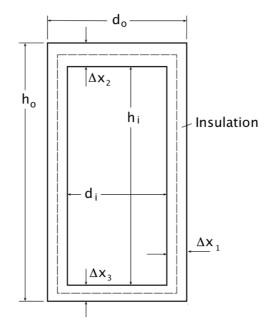
Figure 1. Cross sectional view through an idealised cylindrical tank of inner diameter  $d_i$  and height  $h_i$  covered with insulation of thickness  $\Delta x$ .
