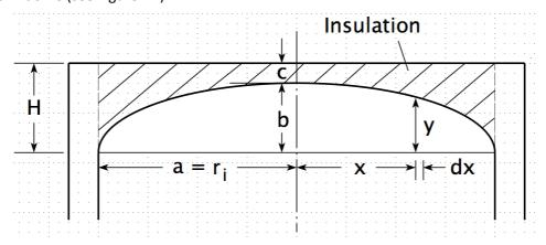
**Figure A2.** Schematic diagram of the top section of a hot water tank with an ellipsoidal dome, where *a* and *b* are one-half of the ellipse's major and minor axes respectively. The average insulation thickness above the tank dome can be determined by calculating the volume of the insulation above the dome and dividing the volume by the circular area below the dome.
